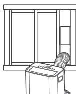
Sliding Window Installation
