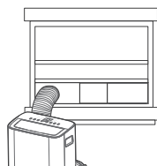
Hung Window Installation
