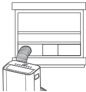
Hung Window Installation
