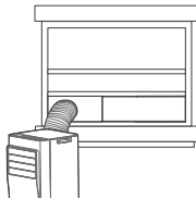
Hung Window Installation
