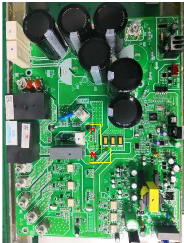
Figure 6-2.3: P and N terminals on Inverter module
