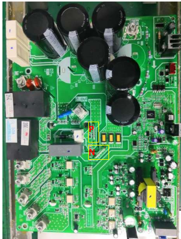
Figure 6-2.4: P and N terminals on Inverter module
