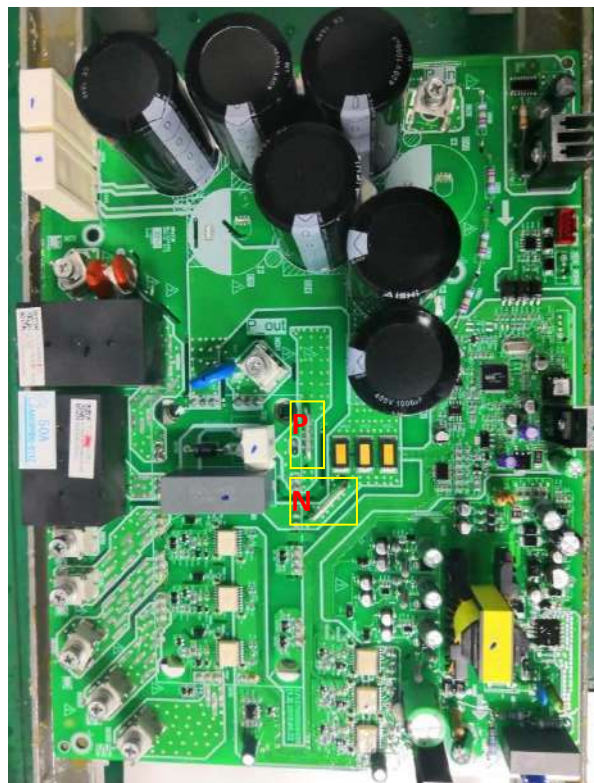
Figure 6-2.1: P and N terminals on Inverter module
