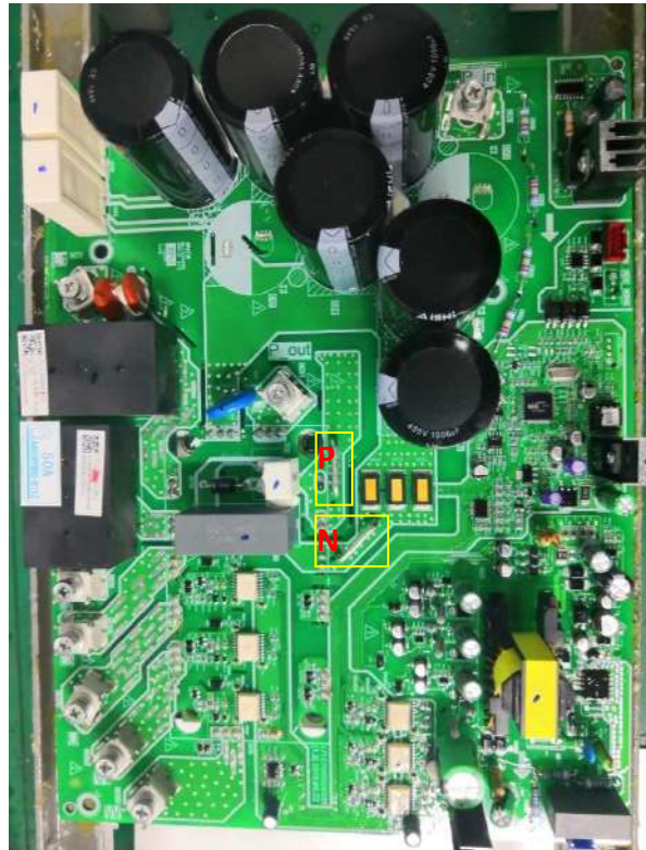
Figure 6-2.4: P and N terminals on Inverter module
