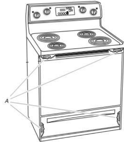
A. The model/serial/rating plate is located on the frame behind a top corner of the door or either side of the drawer.
