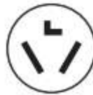
3-wire receptacle (10-30R)
