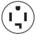
4-wire receptacle (14-30R)
