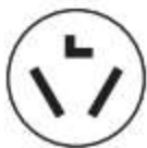
3-wire receptacle (10-30R)
