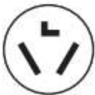
3-wire receptacle (10-30R)
