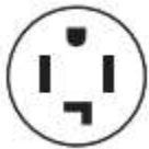
4-wire receptacle (14-30R)
