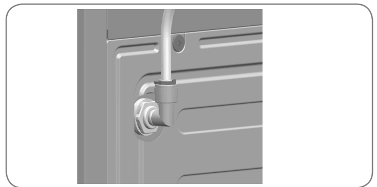
Step 4 ) Install the security clamp.
