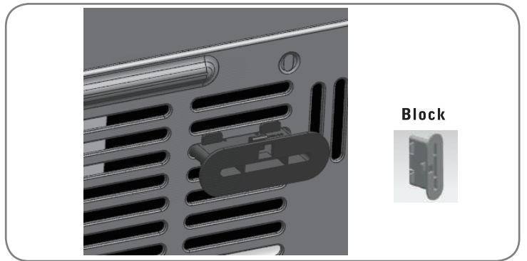
Step 5 ) Install the block.
