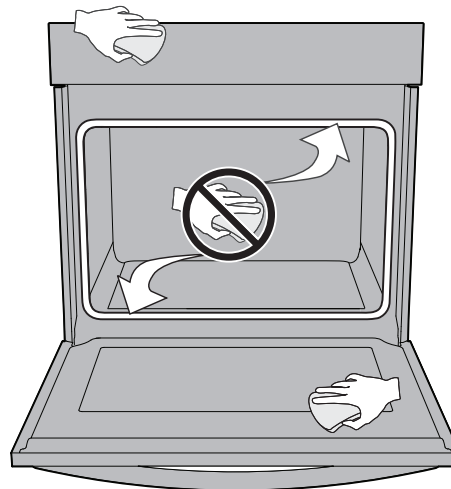
Figure 11: Clean around the oven door gasket
